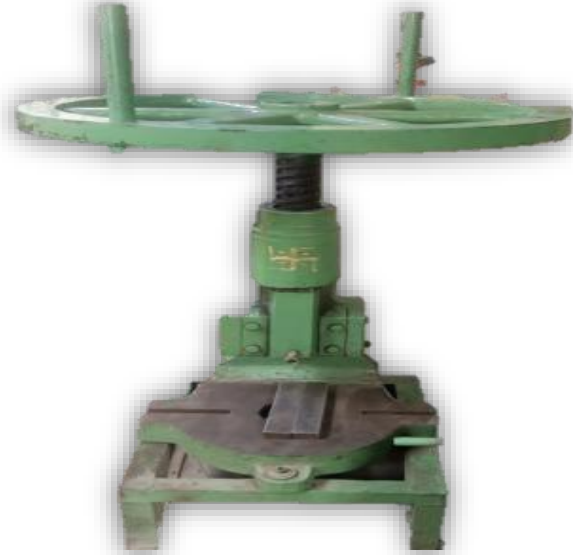
Manual Screw Jack for fitment purpose
